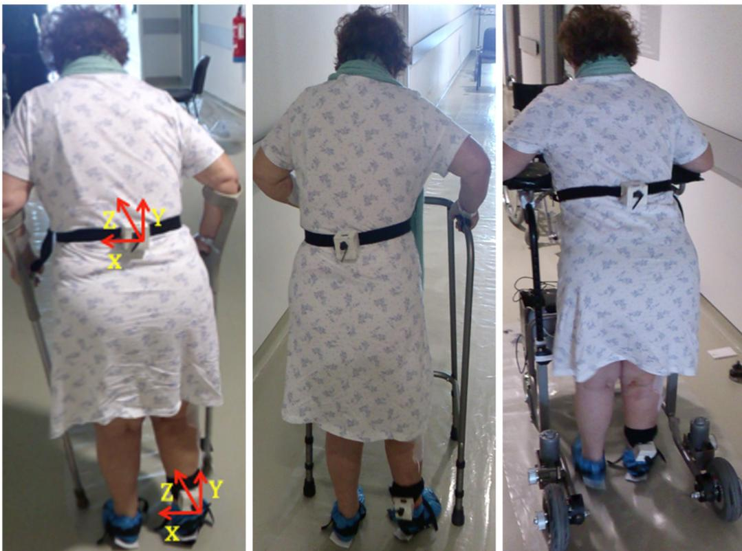
**Figure 2.** Example of the experimental setup with the assistive devices used in this study. Left: Crutches (orientation of the sensors axes indicated); Center: standard walker; Right: RFS walker.
