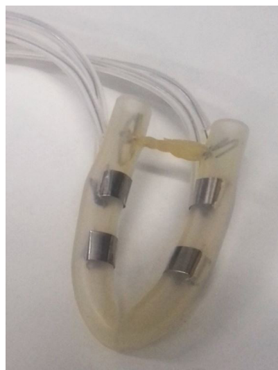
Figure 3. Probe R, with four electrodes.
